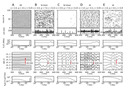
Example network states of the Brunel model with spike raster plot, firing rate, LFP and LFP PSD, A synchronous regular state, B and C synchronous irregular state, D asynchronous irregular state and E asynchronous irregular state
