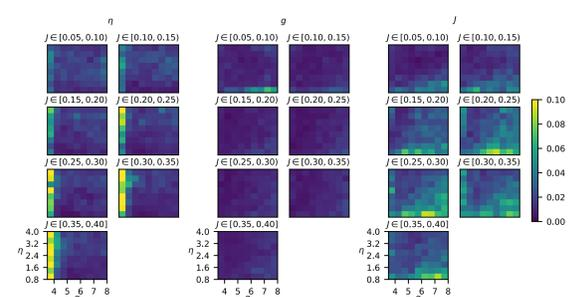
Mean absolute parameter estimation error in different regions of the parameter space, the asynchronous irregular states is predicted with the largest accuracy
