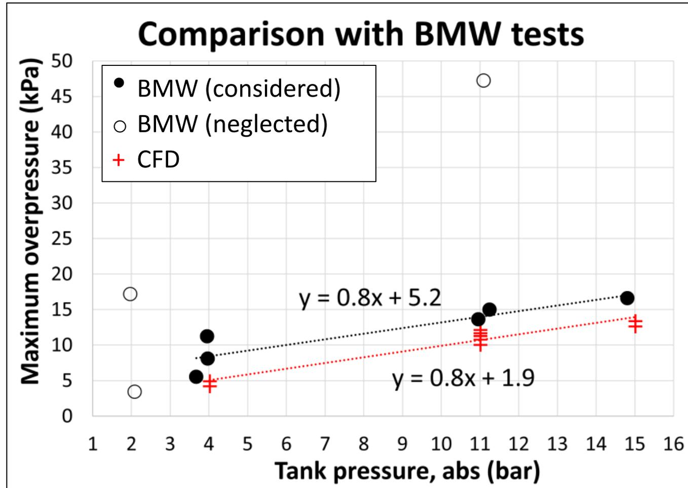
Speculation: the difference in overpressure is caused by the combustion (not simulated)
