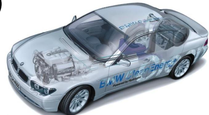
A 7 Series BMW with hydrogen IC engine and LH<sub>2</sub> storage
