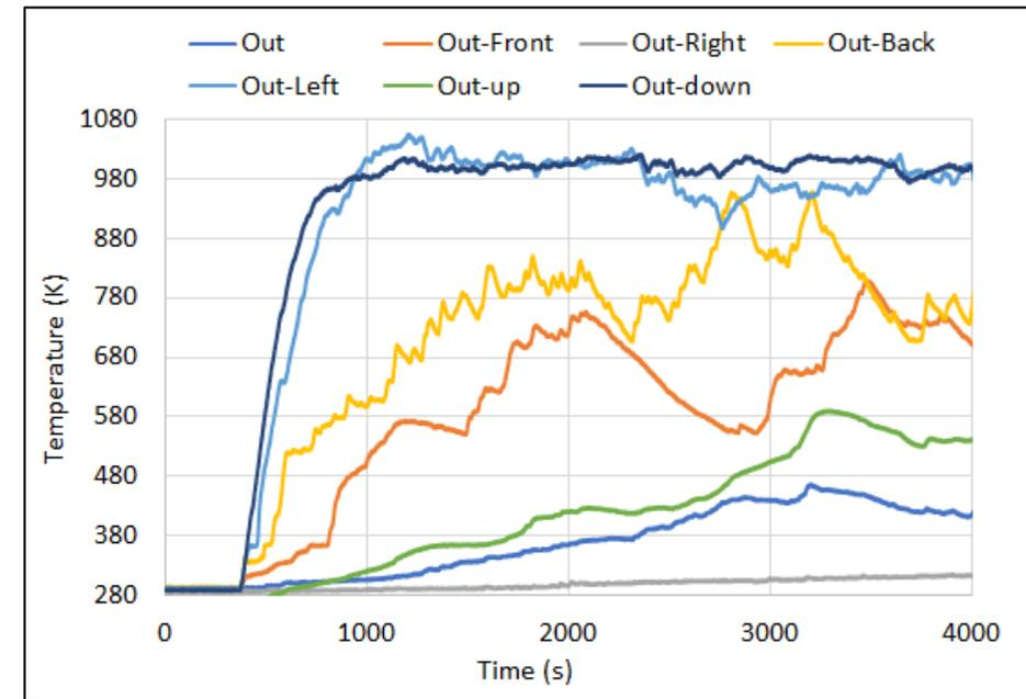
Temperatures measured in different positions on the outer LH2 tank shell during the SH2IFT fire test
