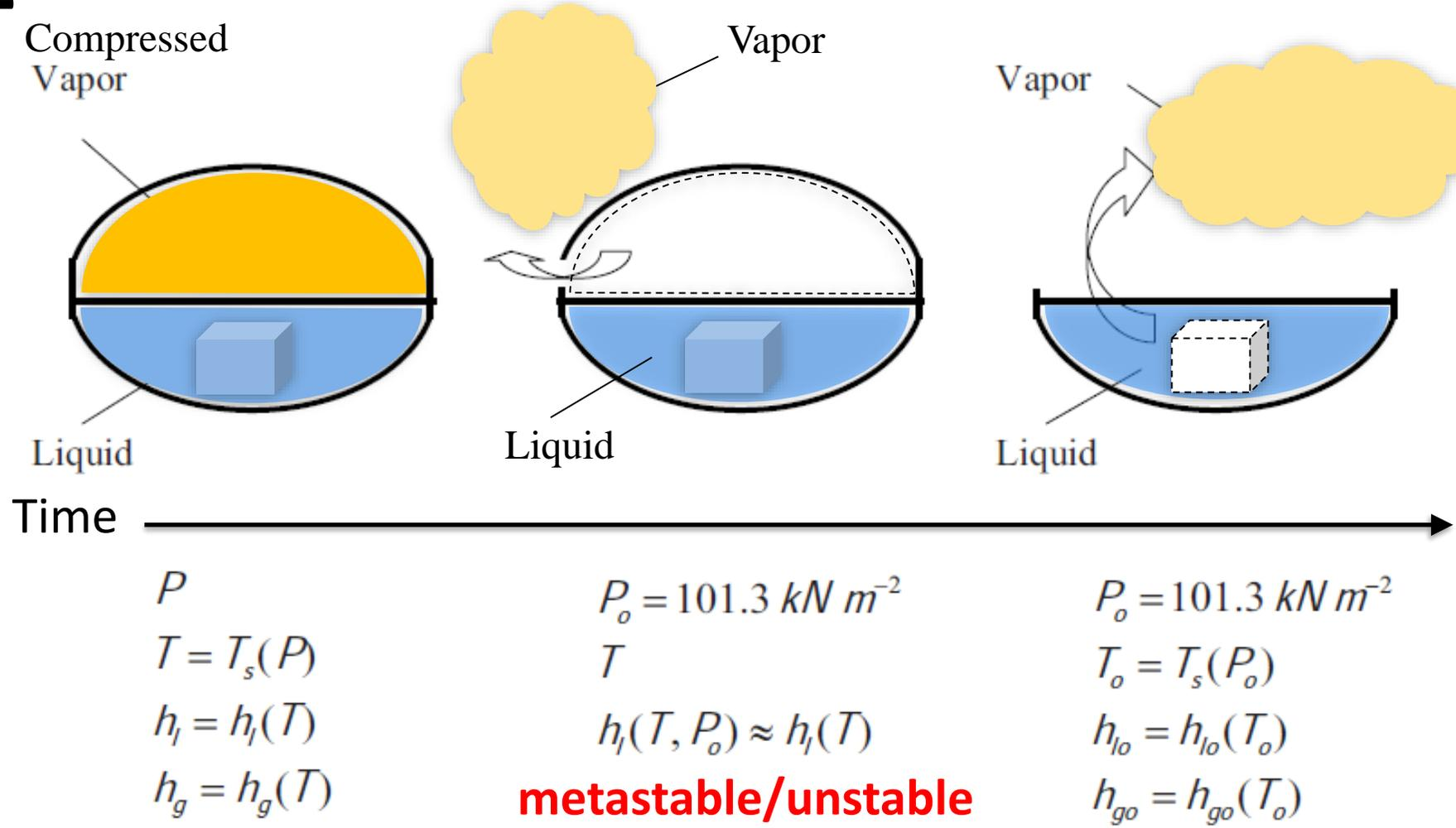
Hot liquid undergoing sudden depressurization in a tank
