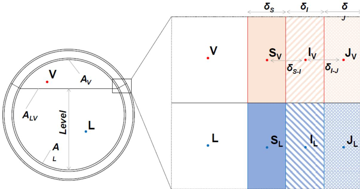
Figure 1: Schematization of thermal nodes discretization. L = liquid phase, V = vapour phase, S = shell, I = insulant, J = jacket,  $A_L$  = liquid wetted area,  $A_V$  = vapour wetted area,  $A_{LV}$  = liquid-vapour interface area.
