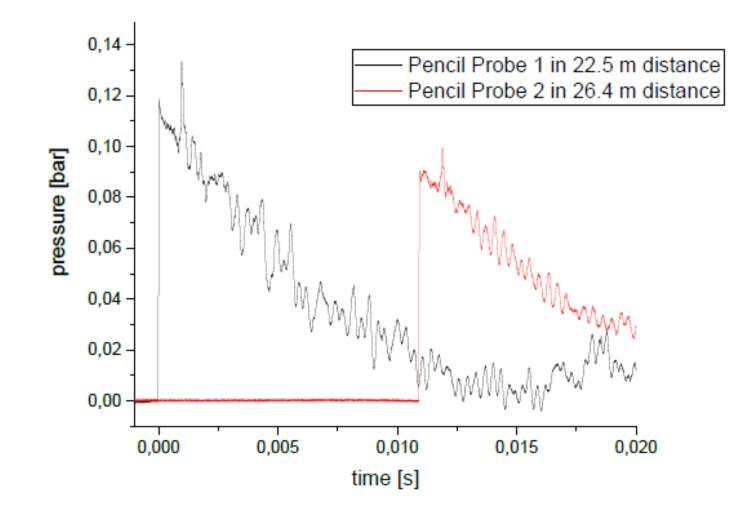
Three peaks: gas expansion, liquid evaporation, combustion
