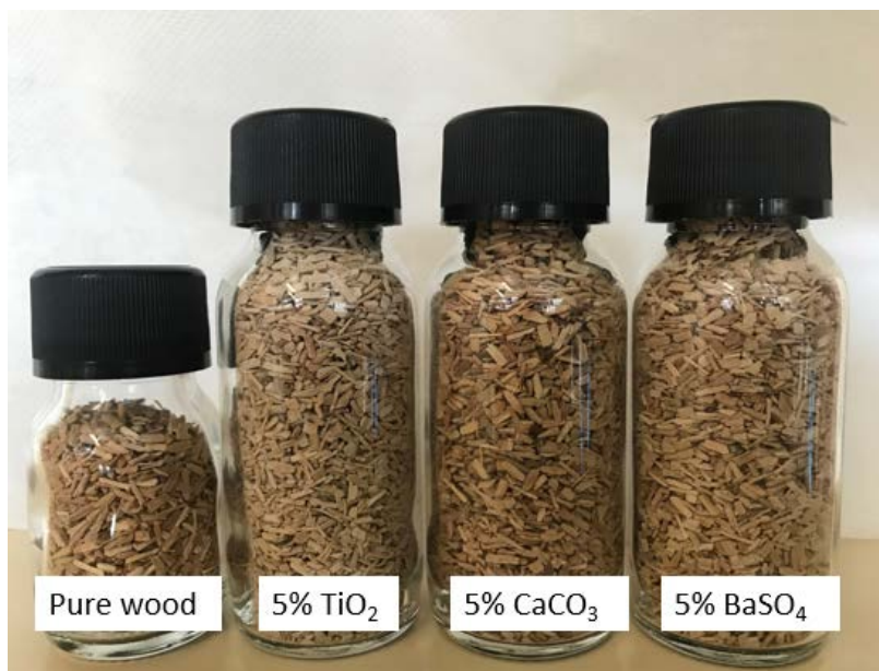
Figure 3.6. Sample preparation: 1h of stirring in rotavapor apparatus (room temperature and atmospheric pressure), Removal of water at 50 °C and 400 mbar, Dry at room temperature at fume hood for 3 days, Water/biomass ration: 750mL/200g (3.75 mL/g), Total contaminated biomass produced: 200g
