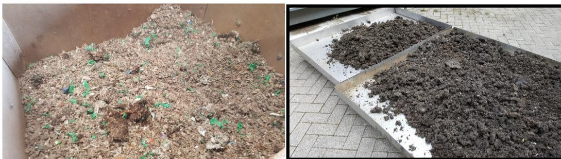
Figure 4. Pre-treatment reject from REG on left side and solids bio-residues from biogas reactors (digestate) on right side.
