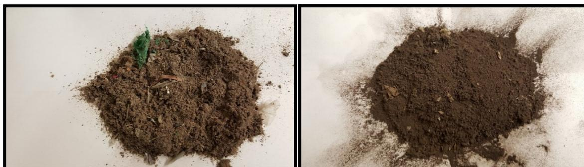
Figure 5. Pre-treatment reject (left) and digestate (right) after drying and grinding.
