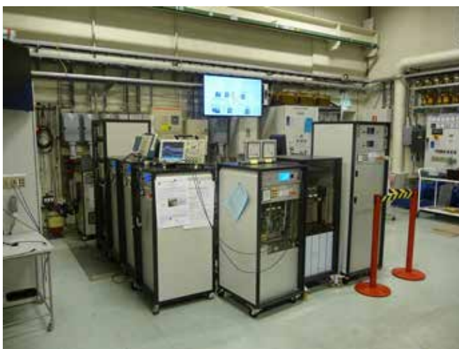
Figure 45: Control of a multi-terminal DC transmission system. Laboratory set-up and experimental results.
