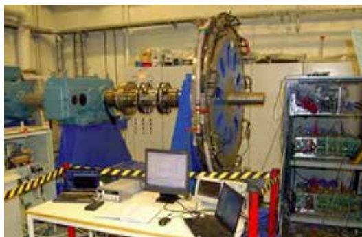
Figure 53: Left: The permanent magnet generator prototype in the SmartGrid laboratory. Right: Diagram illustrating the HVDC generator concept.
