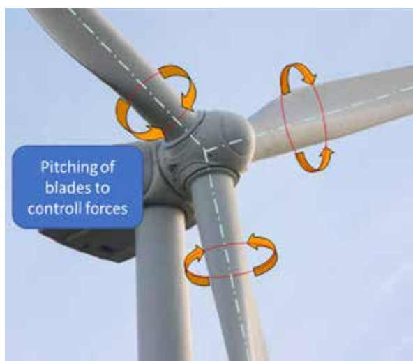
Figure 38: Left: Traditional, motor driven, blade pitching. Right: Diagram showing the bend-twist principle in a blade section.
