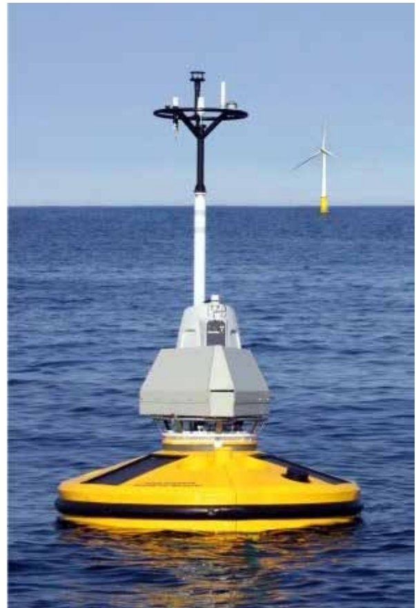
Figure 26: The Fugro Norway floating meteorological ocean buoy that employs LIDAR to measure wind speed at different elevations above sea level.
