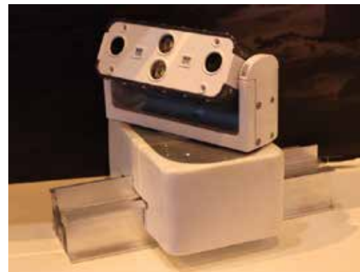
Figure 32: left: A conceptual drawing of a remote presence system installed in a wind turbine nacelle. Illustration: Ø. Netland. Right: A remote inspection high-fidelity prototype.
