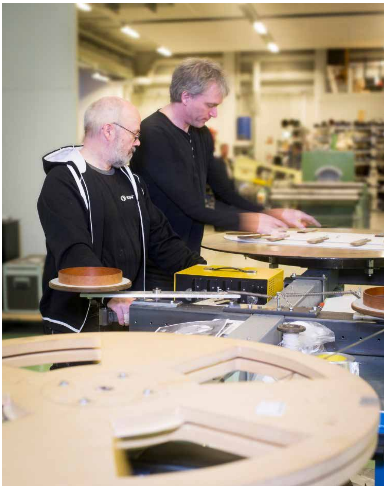
Figure 54: Winding of superconducting test coils for wind turbine generators at SINTEF Energy Research.
