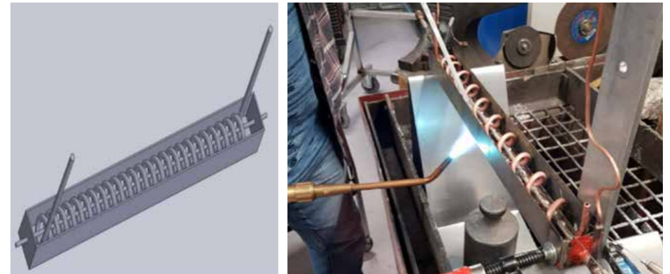
Test section for heat transfer investigation of small tubes.
