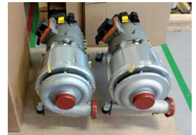
A pair of newly developed oil-free turbo compressors being tested at SINTEF Energy Lab.
