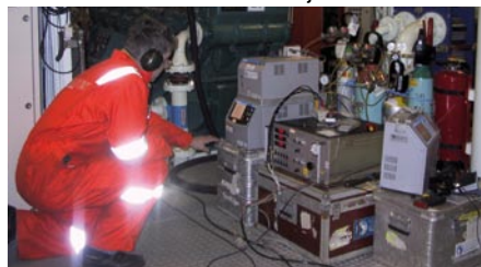
In-field measurement of exhaust gas SCR cleaning efficiency.
