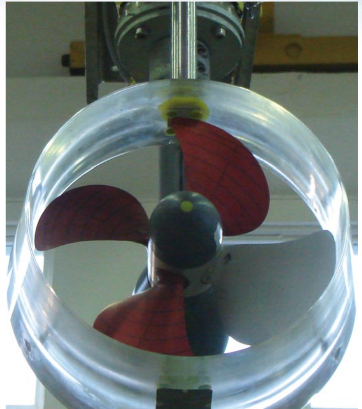
Figure 1. Force measurements on a single propeller blade (grey blade).
