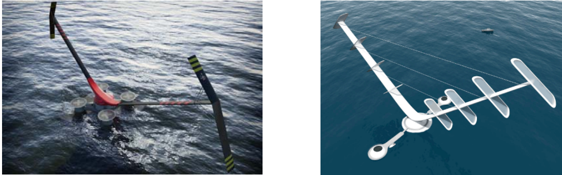
Figure 22: Vertical axis offshore wind turbine concepts from the NOVA project (Source: www.windpower.ltd.uk ; www.nova-project.co.uk )
