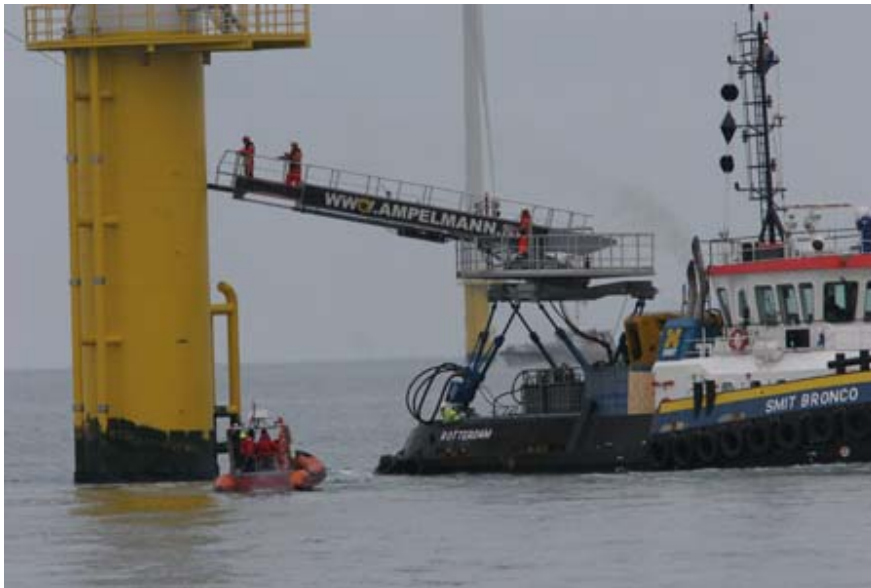
Figure 48: The Ampelmann access system (Source: www.ampelmann.nl )
