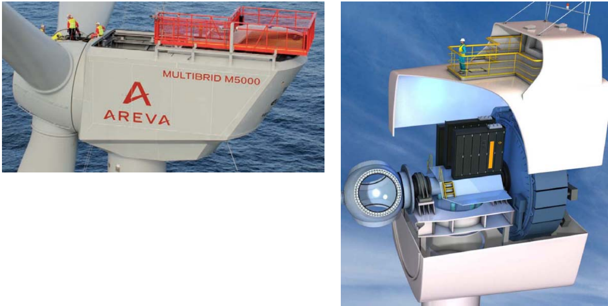
Figure 19: Size of the nacelle of a 5MW wind turbine compared to a person (Source: Multibrid M5000, GE 4.0 - Scanwind)
