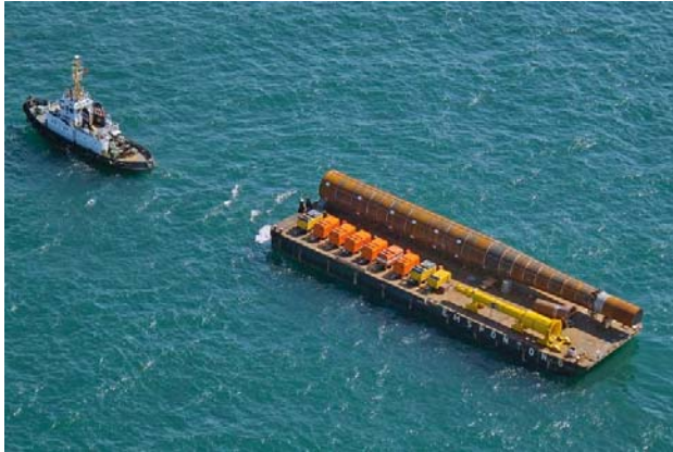
Figure 6: Transport of the monopile for Fino 3 (Source: www.fino3.de )
