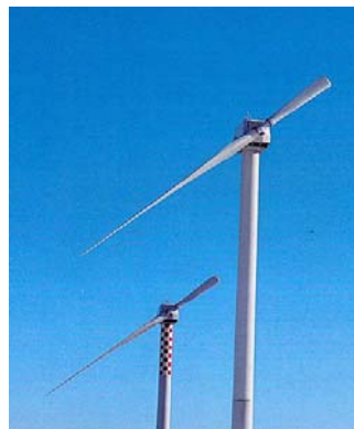
Figure 21: One bladed wind turbine with counterweight (Source: www.wind-energy-the-facts.org )
