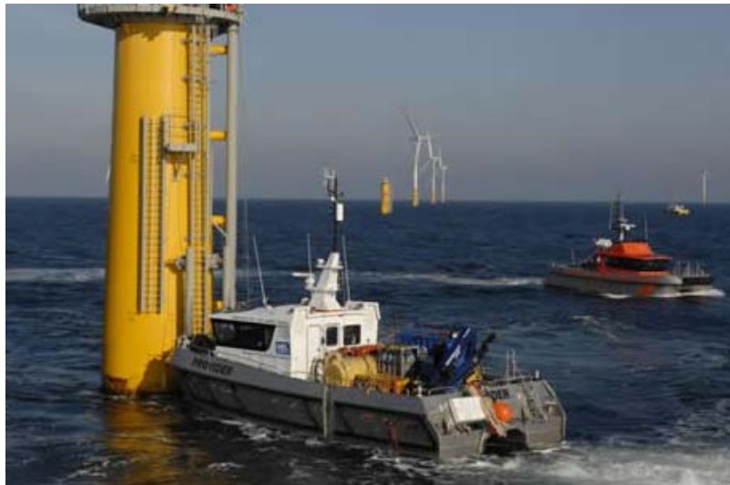
Figure 39: Direct boat landing (Source: www.southboatssp.co.uk )
