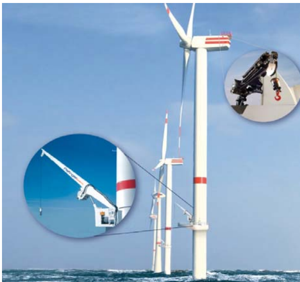
Figure 51: Crane on wind turbine, on working platform or in the nacelle (Source: www.vessel-sales.com )
