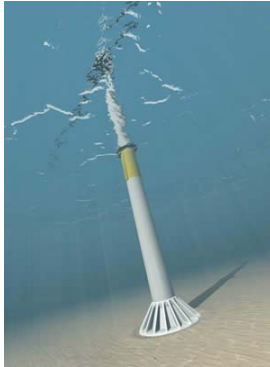
Figure 10: Concept outline of a suction bucket (Source: www.energyengineering.co.uk )
