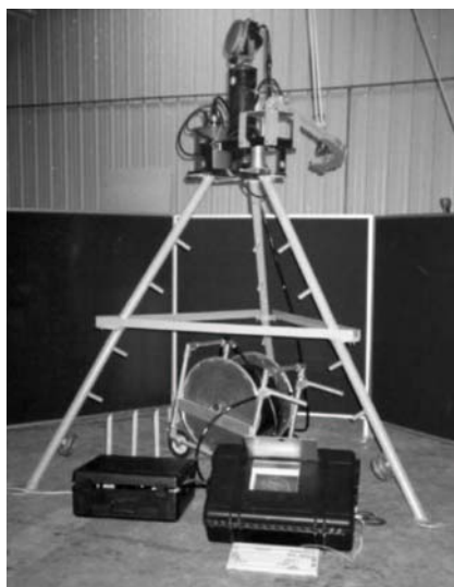
Figur 8 Coastal Structure Acoustic Raster Scanner[18]
