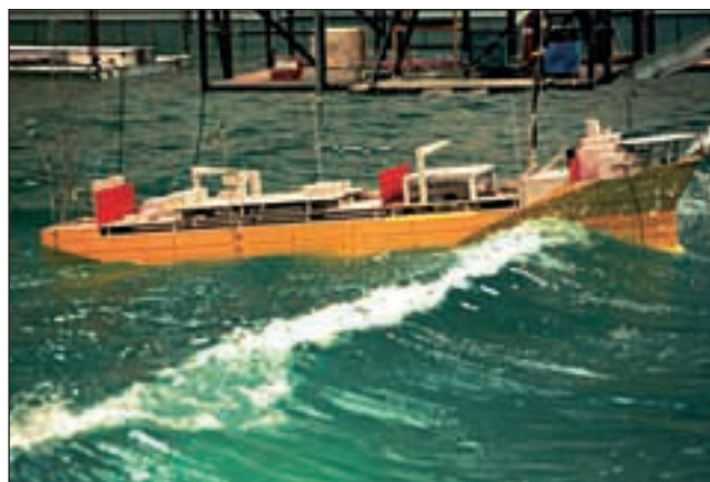
The photo shows the model tests that were performed prior to the development of the Åsgard field. Here, a model of the Åsgard production vessel is being tested.
