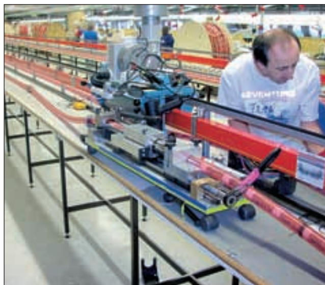
Operator Rune Kalheim secures the proper assembly of a "Q- seabed" sensor casing.
