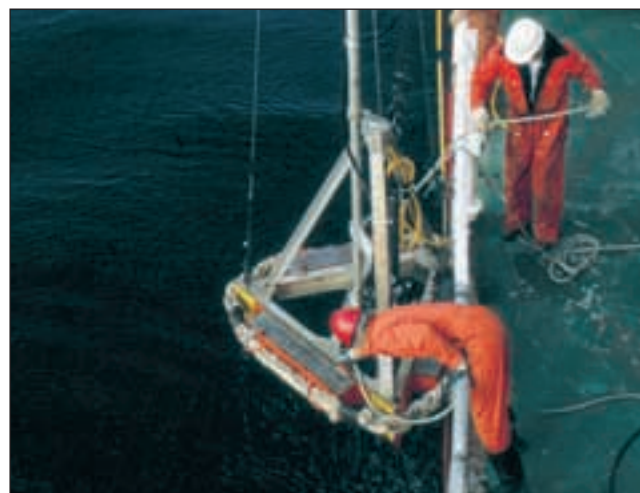
Remotely controlled mini-drilling rig used in the 1980ies.
