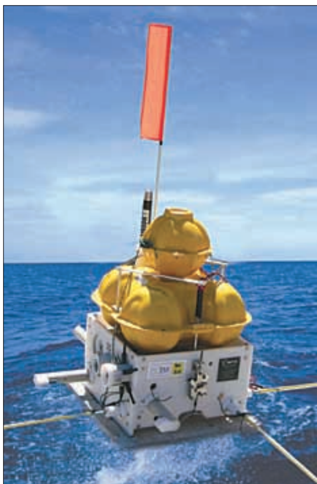
The SBL receiver deployed on the seabed to register low-frequency electromagnetic signals.
