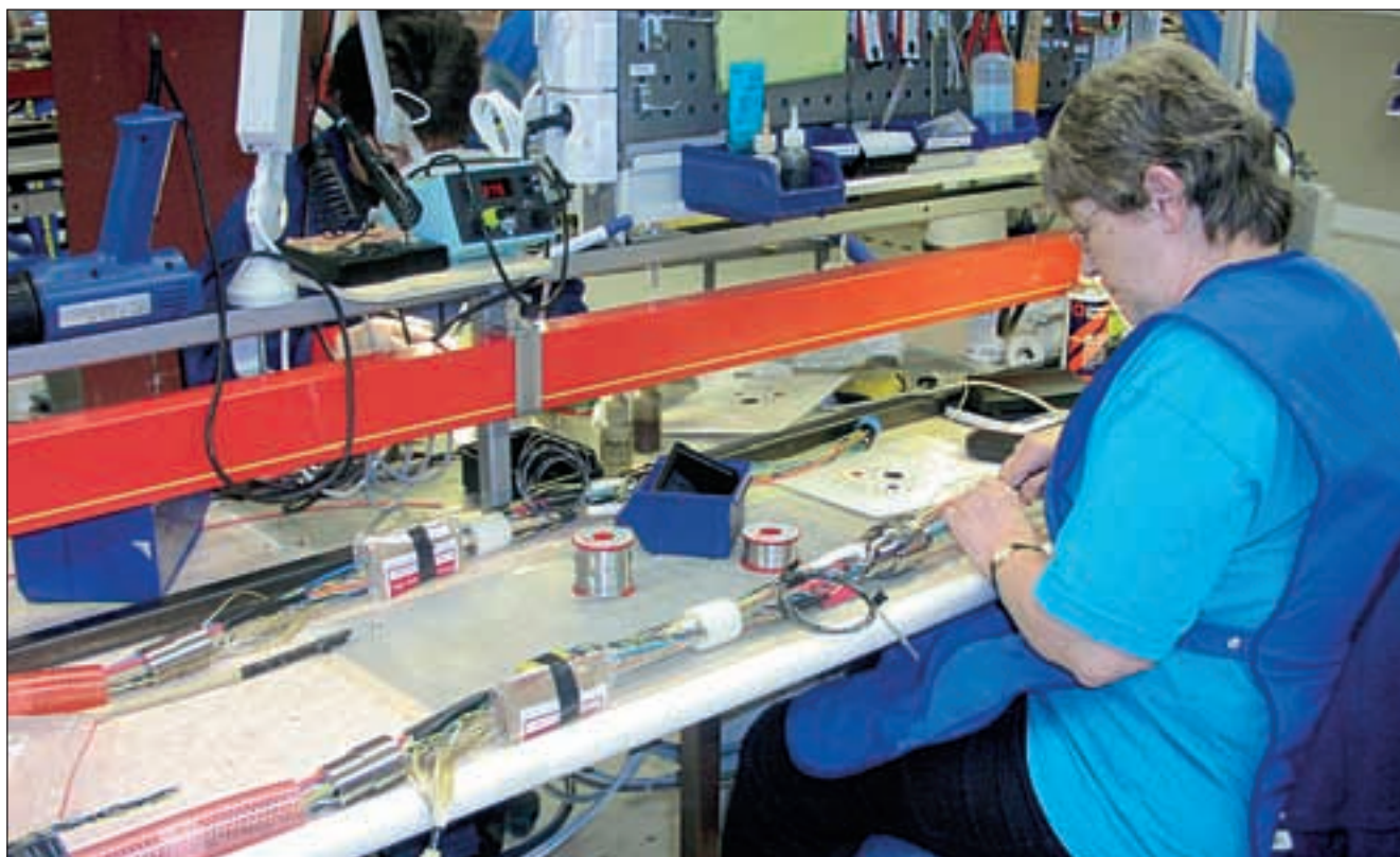
Operator Norma Lærdal of Fjord Instruments in Knarvik near Bergen accurately assembles the combined fibre/electric terminal coupling of a "Q-seabed*" section.
