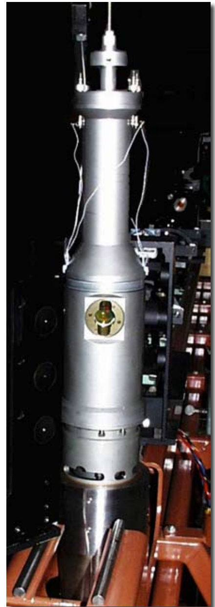
Laser-light scattering cell (shown without surrounding thermostat bath). The (red) laser beam can be seen exiting the cell.
