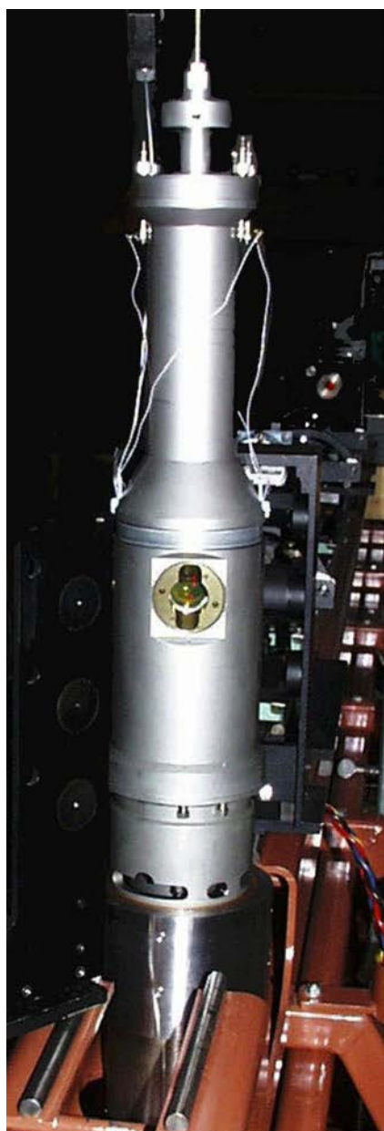
Laser-light scattering cell (shown without surrounding thermostat bath). The (red) laser beam can be seen exiting the cell.
