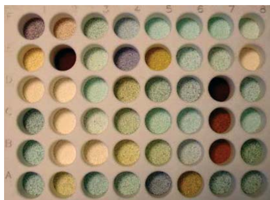
Figure 2 Array of samples ready for parallel testing under high temperature reaction conditions.
