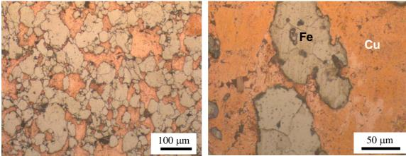
Figure 8. Distribution of Fe particles in Cu Figure 9. Iron powder particles in copper matrix.
