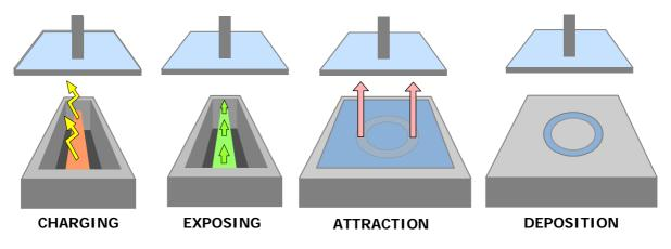
Figure 1. A schematic illustration of the process steps during layer fabrication.
