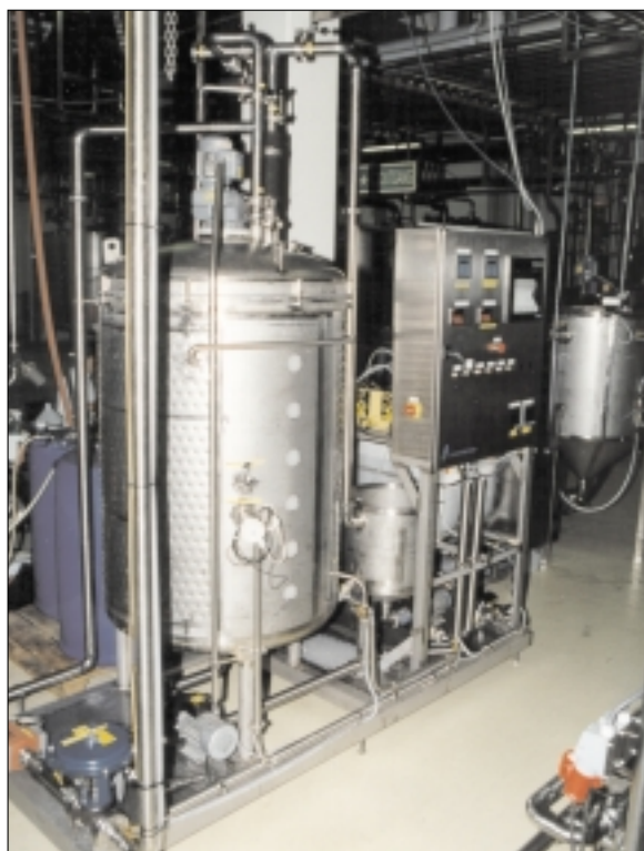
Picture right: Immobilised lactic acid bacteria are used in a combined biological and chemical purification of dairy waste-water leading to production of high quality animal feed.
