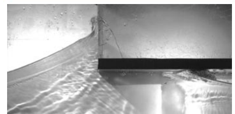
Wave-on-deck problem: schematic (upper), and simple experiment (lower).
