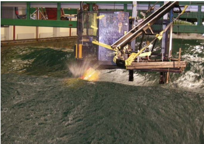
Photo 1: "Forward Distance" model tests in bow oblique seas (Regular Wave H=11.3 m and wind 35 m/s).
