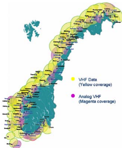
Figure 2. Coverage map of TMRs Digital VHF system ('VHF Data').
