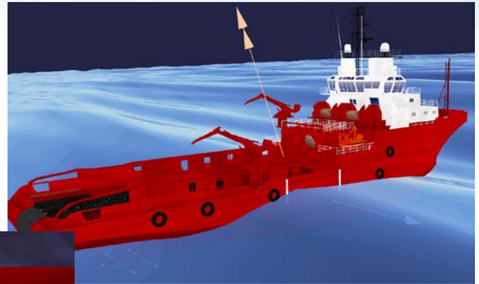
Snapshot from SimVis showing a VeSim simulation of a supply vessel in a seaway. The arrows can show various forces and moments acting on the vessel and offers the end users and developers an excellent way of checking and understanding the physics in the numerical models as well as being a tool for communicating complex results to people from other disciplines.
