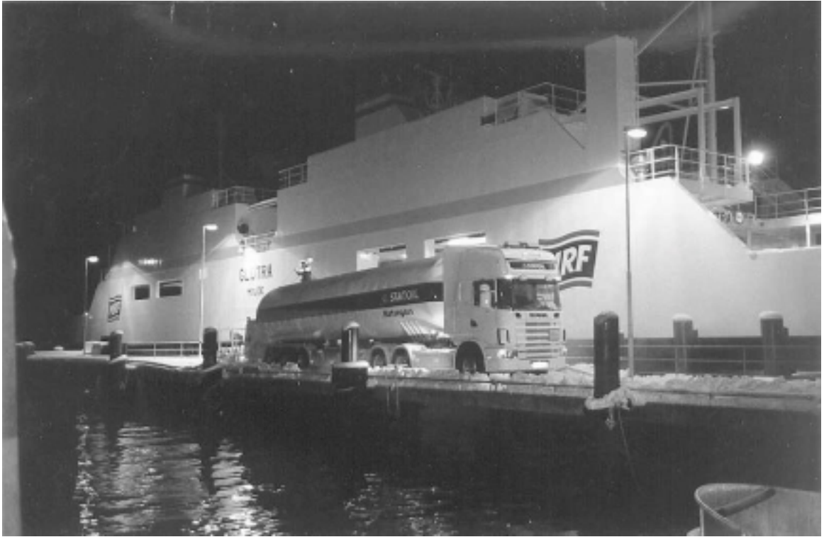
Figure 3. Refuelling LNG directly from the truck during docking at night.
