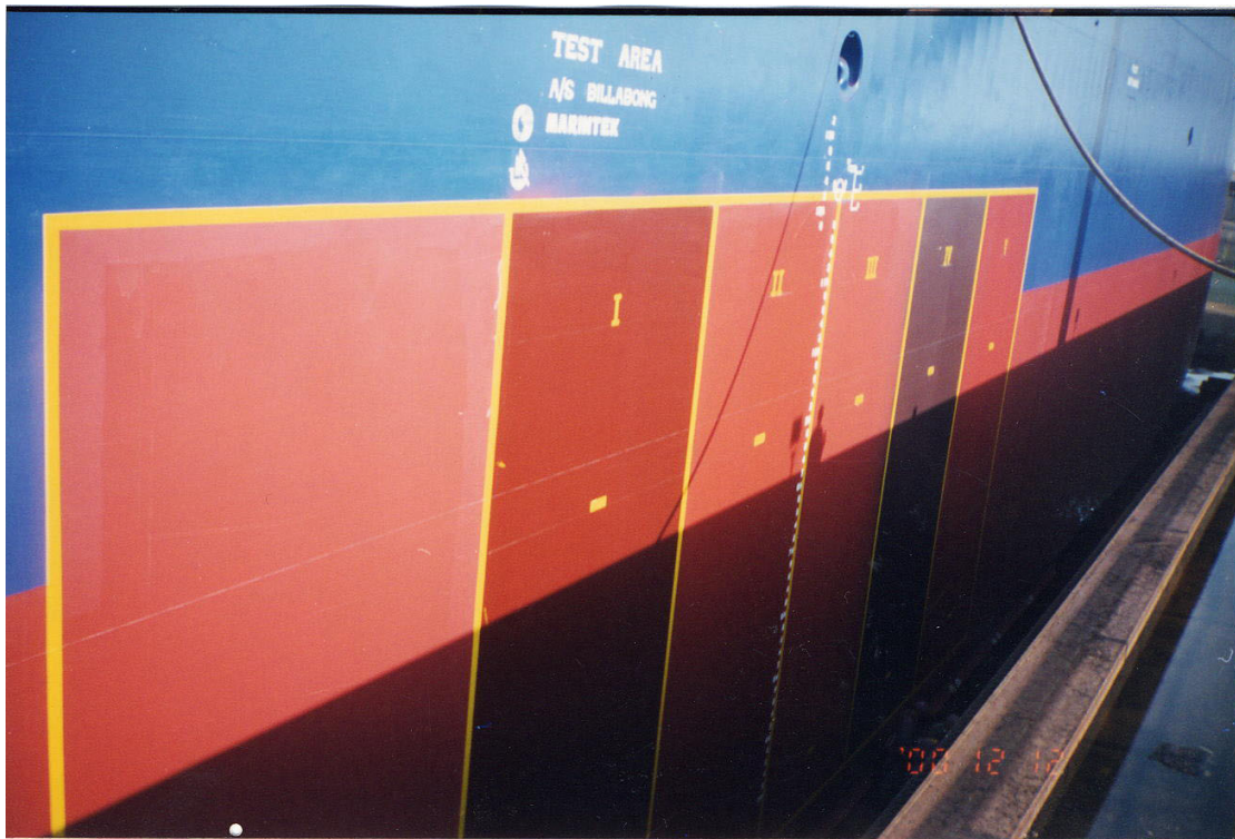
Figure 7: Test patch layout, MV “Star Harmonia”
