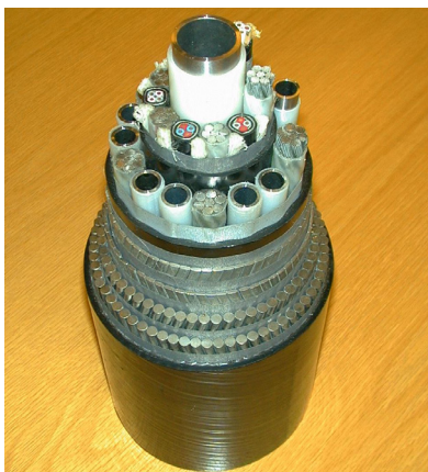
Figure 1. A typical umbilical cross-section, the Norne dynamic CSU (Control and Service Umbilical), installed in 1996.
