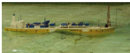
Ku Maloob Zaap - Mexico's first FPSO.
