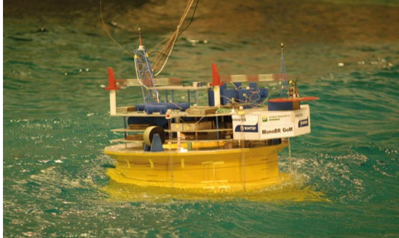
MonoBR, a single column floater for Gulf of Mexico. From tests in the Ocean Laboratory.
