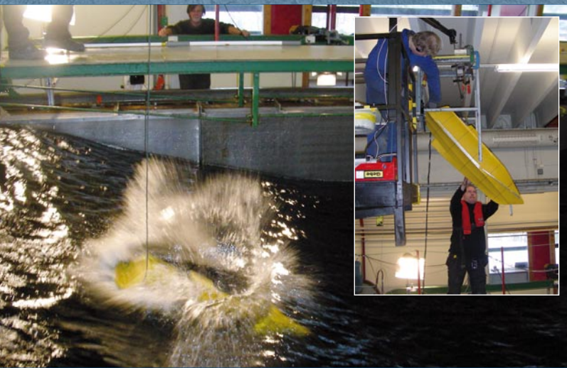
Testing of lifeboats under various wave conditions.
