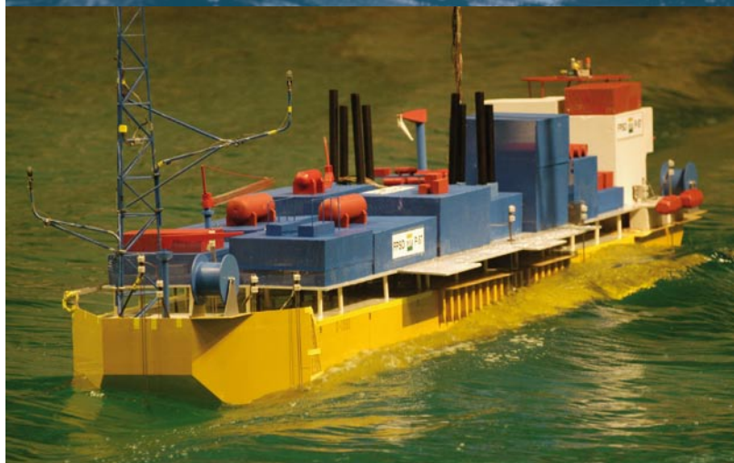
P-57 FPSO-BR, model tests for Petrobras.
