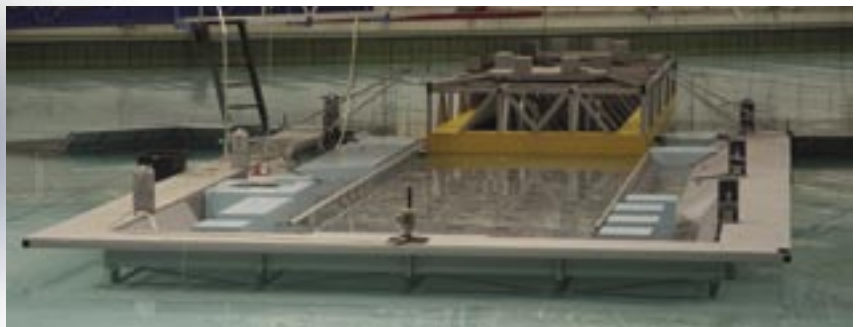
Model testing for Statoil - docking a process barge for the Snøhvit project on Melkøya.
