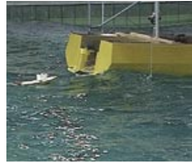
Model tests in the Ocean Basin for the US Coast Guard, showing rescue boat entering and leaving the stern port.
