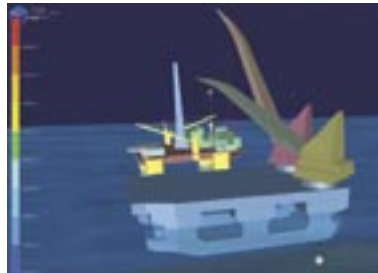
A heavy lift operation being tested by means of models and simulator.
