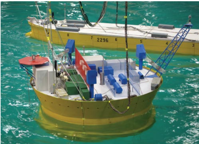
150 DWT export tanker moored to Sevan 1000 FPSO for offloading.
