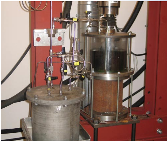
Test rig for corrosion fatigue testing of armour wire for flexible pipes.
