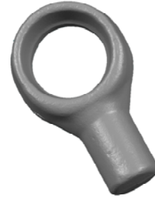
Figure 2: 3D model of the car part obtained by stitching together six 3D images taken from different angles of the component.
