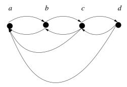
Figure 2: A chain of trust promises to transfer some valuation of trust in one direction (only), from node a to each agent up to node d. This method is unreliable because nodes b and c are under no obligation to pass on the correct value. Note that these are promise arrows, not trust arrows.
