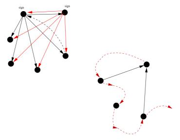
Figure 6: In a web of trust an agent signals a promise to all other agents that it has trusted the authenticity of the originator's identity. As a key is passed around (second figure) agents can promise its authenticity by signing it or not.
