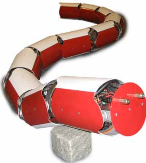
Figure 1: Anna Konda – the world's biggest and strongest snake robot. Multi-joint robots offer great traversability, but also numerous challenges in modeling, design and control due to a large number of interconnected links and complex dynamics.
