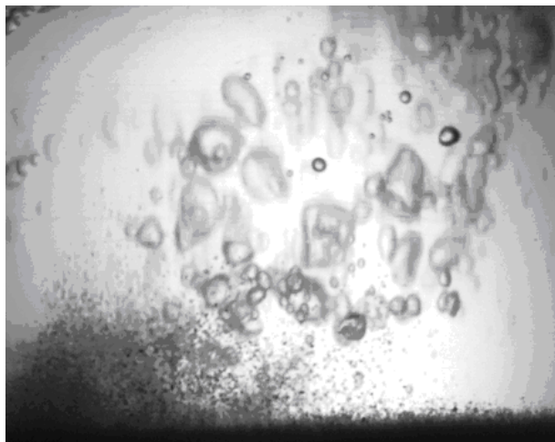
Figure 1: Sand transport in horizontal air-water slug flow showing entrainment of sand in the middle of a slug body. Sand particle diameter was 280 \mu\text{m} . Pipe diameter was 67.2 mm (Reference: experiment be03122 of SINTEF Petroleum Research project 32103200).
