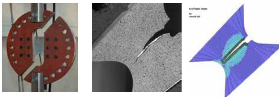
Figure 4: Arcan test set-up in the laboratory (left) and crack propagation in test (middle) and simulation (left) for 45° load angle. Damage-driven adaptivity is used in the simulation.
