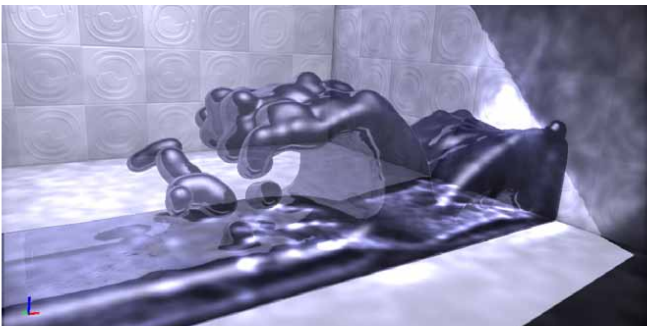
Figure 1: Simulation of sloshing using smoothed particle hydrodynamics implemented on GPUs.
