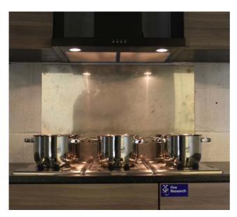
We have a test set-up ready for standard type testing of kitchen stove guards according to the new prEN 50615 "Particular requirements for devices for fire prevention and suppression for electric hobs (cooktops)".
