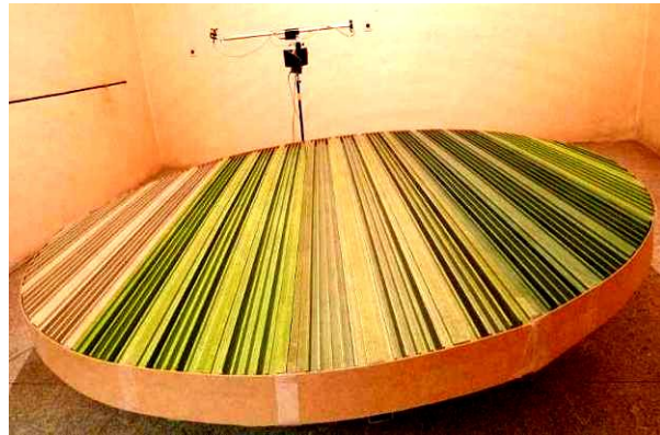
Figure 4. Sample of diffuser in reverberation chamber
