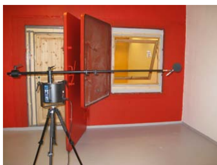
Foto 1. Window mounted in the test laboratory.
