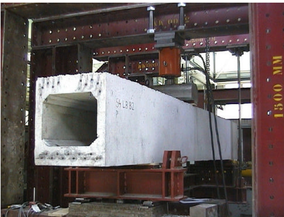
Figure 38 Test arrangements for the shear test
