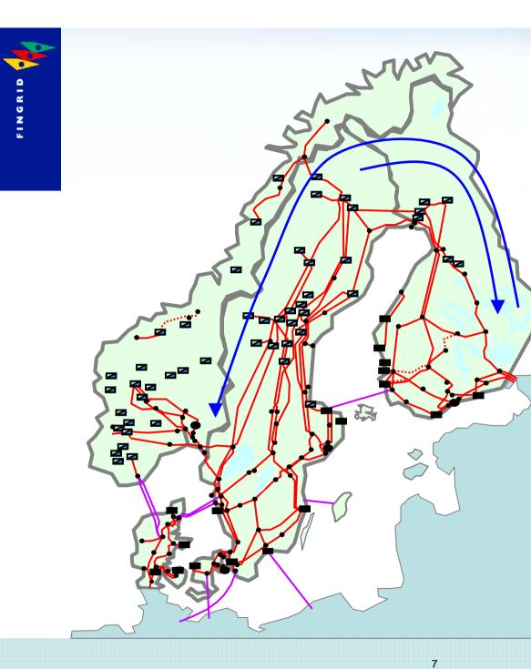
Voltage stability gives transmission limits when importing, lowfrequency damping when exporting
