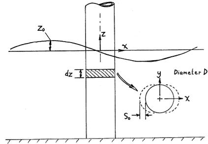
Find the net force of the fluid on the structure,  $F(z, t)$ .
