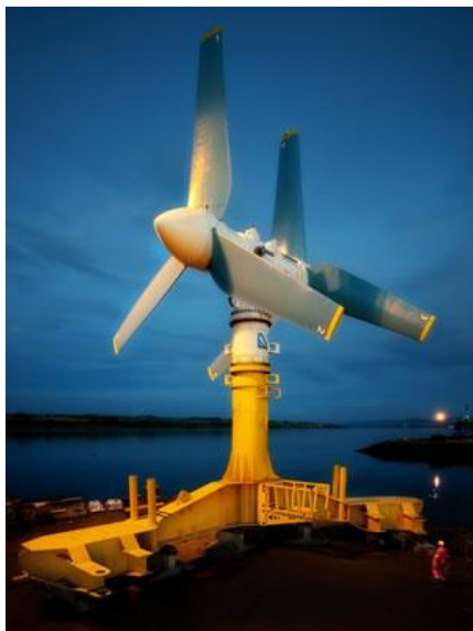
1.1 MW tidal turbine of Atlantis Resource Corporation (delivered)
