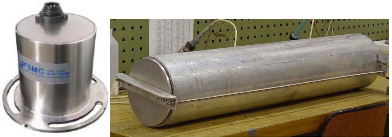
Figure 2.4 The SMC S-108 sensor and the steel tube it was mounted in during the fieldwork
