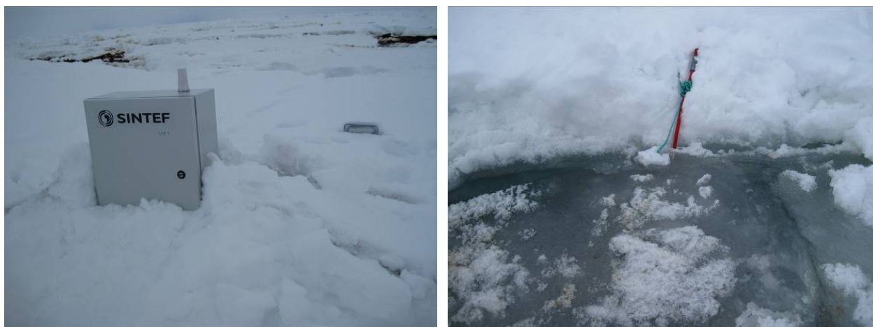
Figure 2.9 The control box containing batteries, data logger and control unit for the submerged UVF sensor. The UVF antenna can be seen on top of the box.
