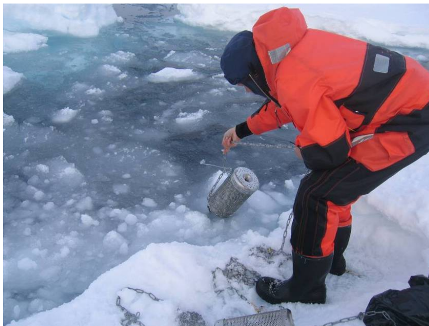
Figure 2.13 Deployment of SPMD into the water
