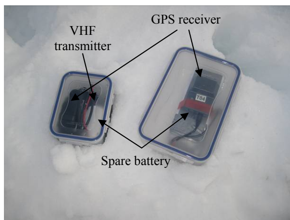
Figure 2.6 GPS Garmin and Trackstick systems placed on the ice for testing before the oil release. The Trackstick unit is marked with T4 (in right box).
