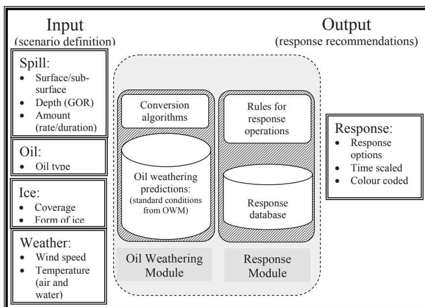
Figure 10.1 - Basic architecture of the OSRG system
