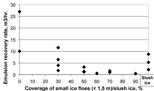
Figure 7.3 -Calculated recovery rates as a function of increased coverage of small ice floes
