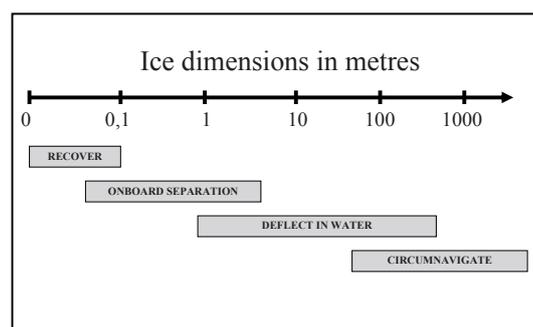
Figure 7.1 - Main ice processing principles roughly related to ice dimensions (metres)
