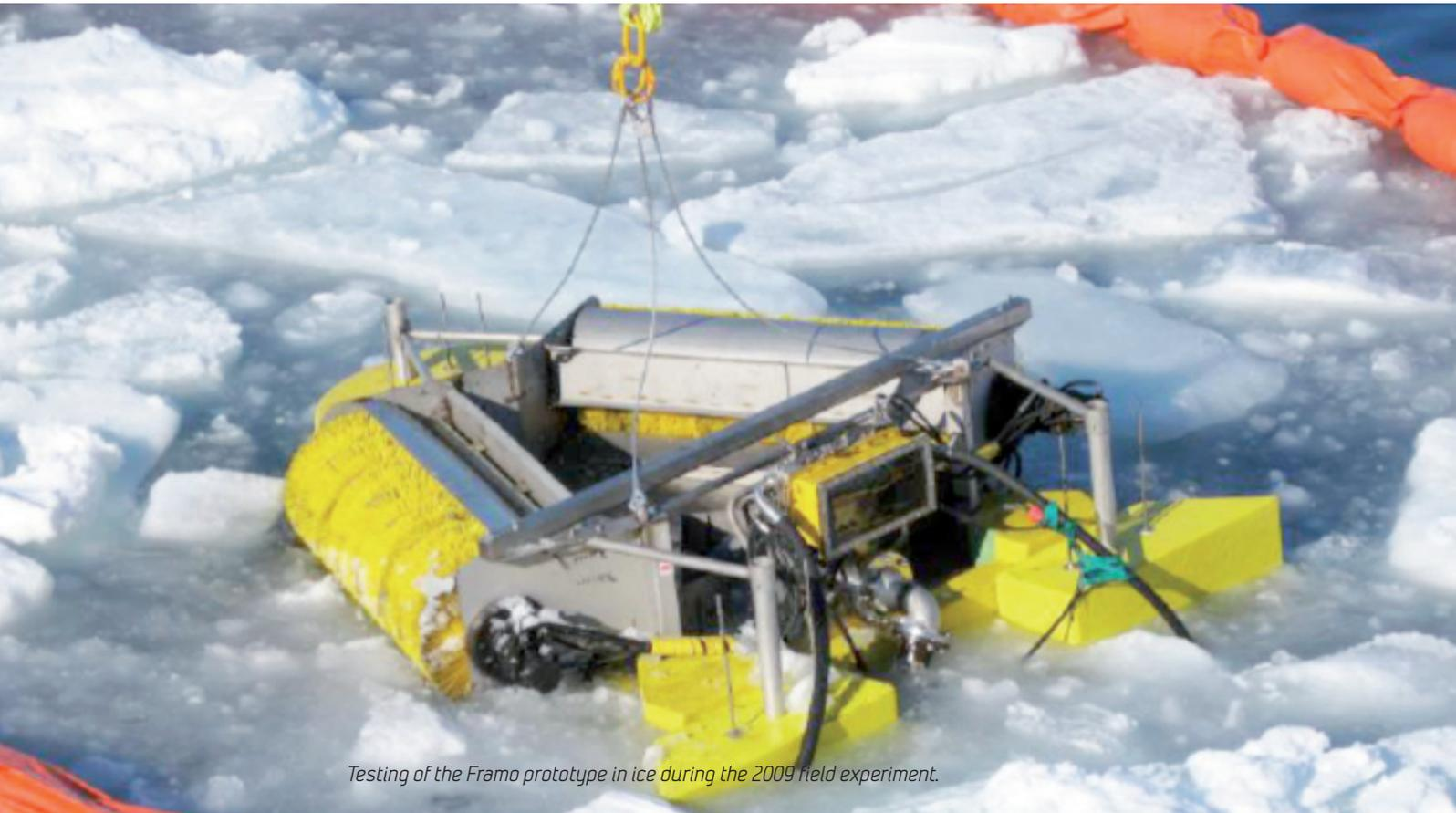
Testing of the Framo prototype in ice during the 2009 field experiment.
