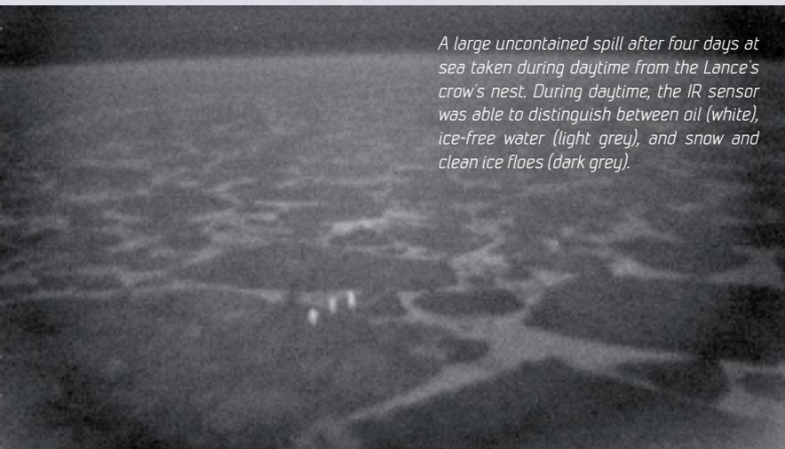
*A large uncontained spill after four days at sea taken during daytime from the Lance's crow's nest. During daytime, the IR sensor was able to distinguish between oil (white), ice-free water (light grey), and snow and clean ice floes (dark grey).*
