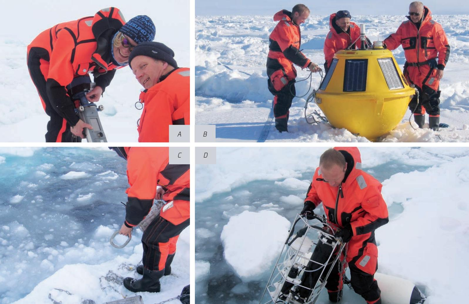
Fig. 9.2 - Examples from FEX 2009 measurement program A) Seaguard - current measurements B) Mini Seawatch - waves in ice field C) Deployment of SPMD D) Deployment of KISP
