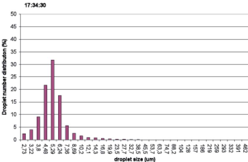
Figure 6.3 - Droplet size measurements document that the oil is broken down into small particles (5-30 um) with extremely low rising velocity
