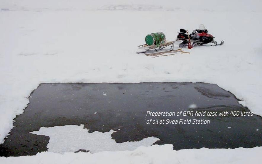
*Preparation of GPR field test with 400 litres of oil at Svea Field Station*
