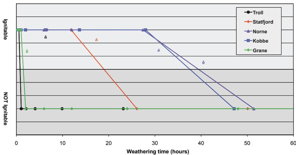
Figure 5.2 - Ignitability measured with the laboratory burning cell as a function of weathering time for the five different oil types used in this study. All were measured at 50% ice coverage.
