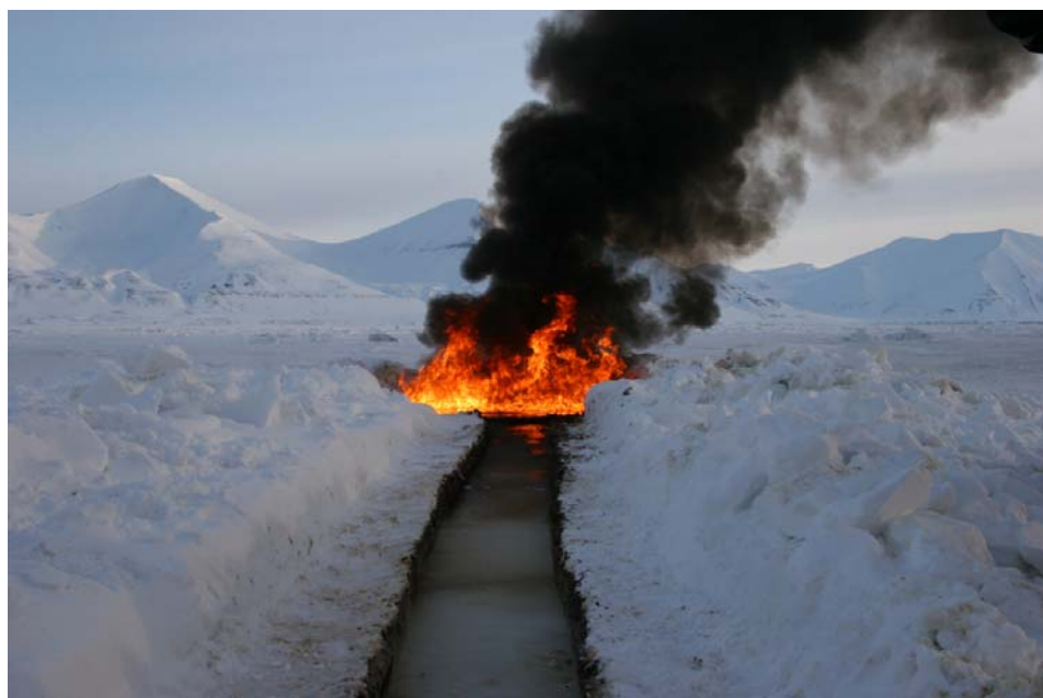
Figure 4.10: In situ burning of weathered oil. The system consists of a burning basin connected to the weathering basin with a channel (see earlier figure) in operation.
