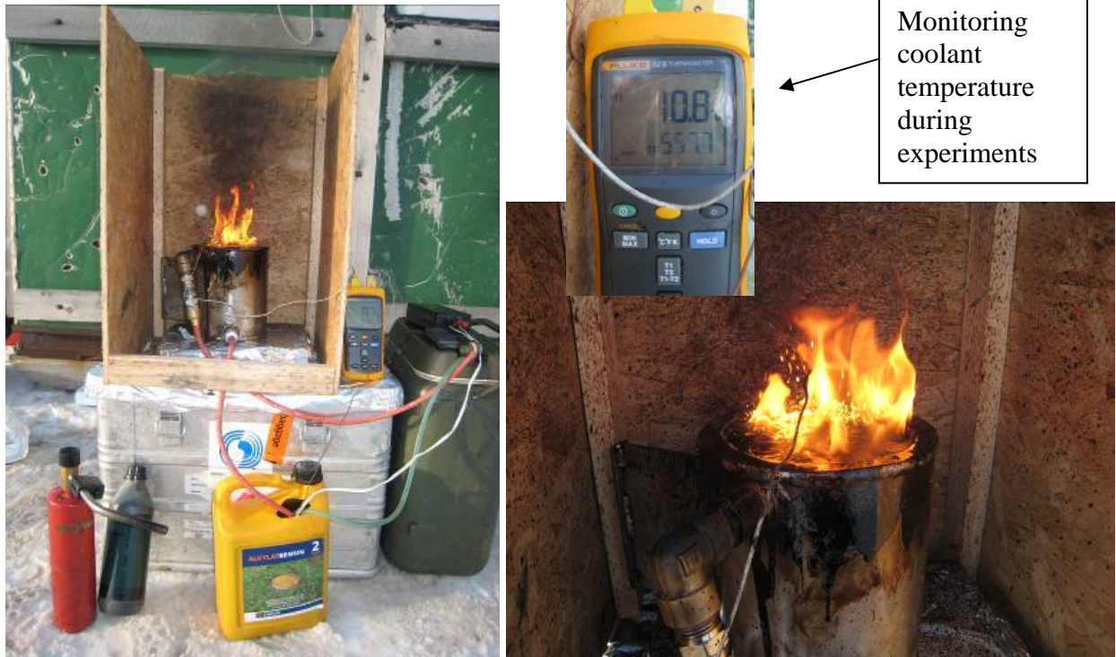
Figure 4.12: The core unit of the laboratory burning cell operated in “field mode”. Only the cell itself, the butane igniter, the cooling unit (pump, coolant and thermos), and the flame temperature unit/logger were operated in the field.
