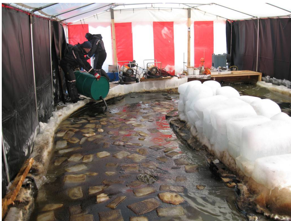
Figure 4.3: Overview of the meso-scale basin cut out in the first-year fjord in Svea, Svalbard. The tent was used to control the air temperature and ice conditions.
