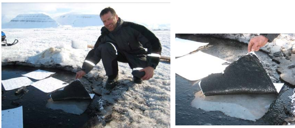
Figure 4.11: Collection of residue. After cooling, the residues were easy to remove/collect with 3M adsorption pads. Quantitative collection of residues was important for determining burning effectiveness.
