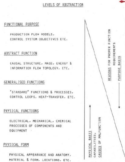
Figure 4. The abstraction hierarchy used for representation of functional properties of a technical system.
