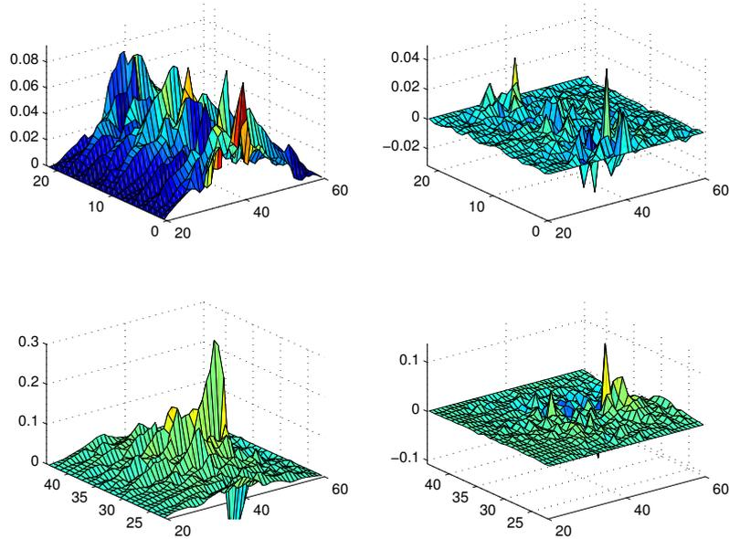
Fig. 2. The  $x$ -component (left) and  $y$ -component (right) of two MMsFEM base functions for a two-dimensional model with random coefficients using the boundary conditions defined by (17) and (19). The top base function corresponds to an interface away from the near-well region while the bottom base function corresponds to a well-block interface.
