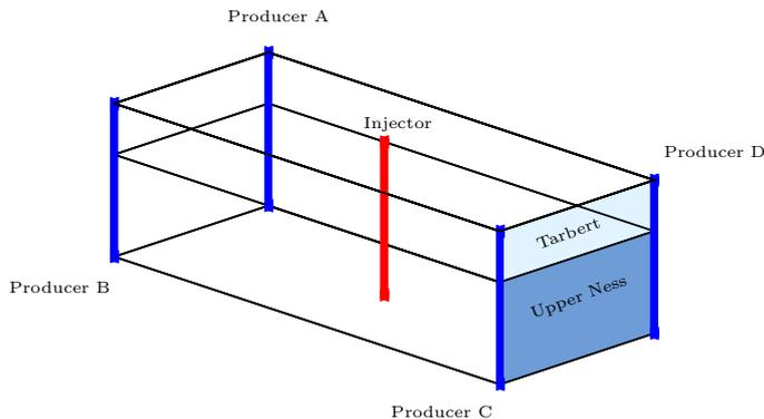
Fig. 3. Well configuration for reservoir model used in the tenth SPE comparative solution project. The model dimensions are  $1200 \times 2200 \times 170$  ft, and the fine and coarse meshes consist of  $60 \times 220 \times 85$  and  $5 \times 11 \times 17$  grid cells, respectively.
