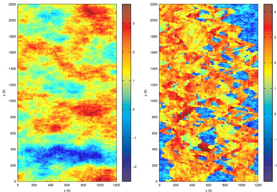
Fig. 4. Logarithm of horizontal permeability for layers in the Tarbert (left) and Upper Ness formations (right).
