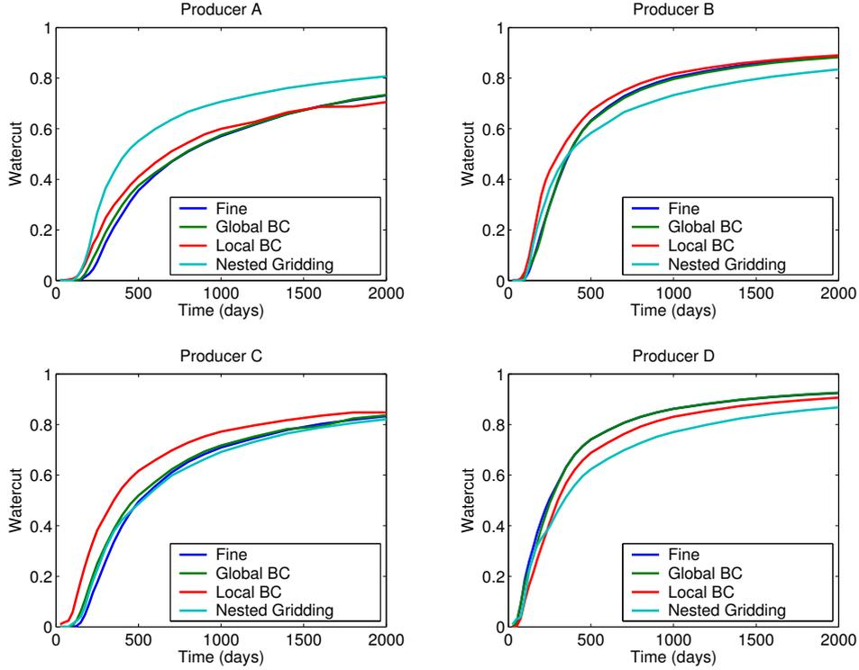
Fig. 6. Watercut curves for the full three dimensional SPE 10 model.
