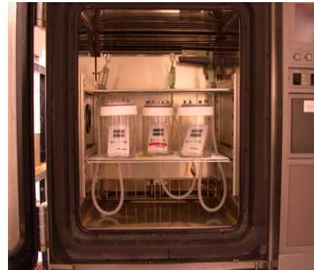
Testing of electrodes and biomaterial coatings (polymers, parylene,  $\text{TiO}_2$ , ...)
