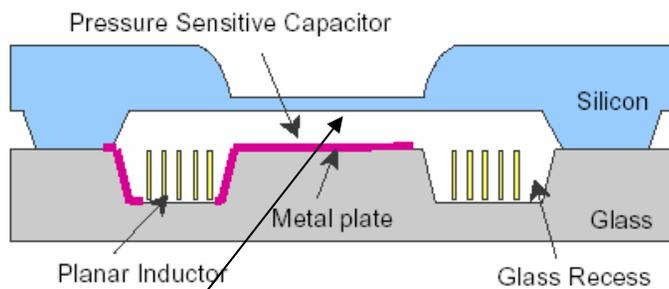
6  $\mu\text{m}$  silicon membrane
