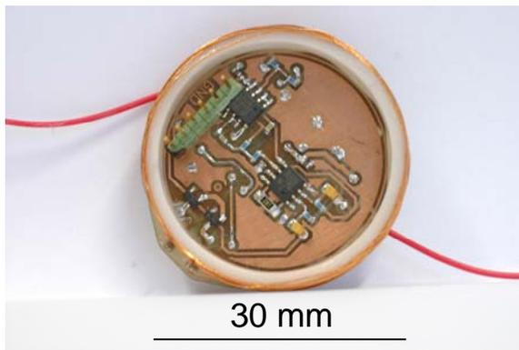
Prototype with a coil antenna
