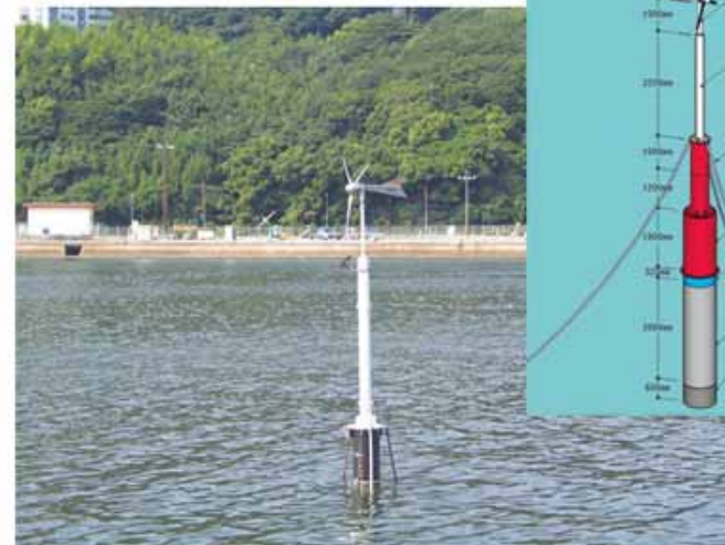
Scale model of Spar type: Prof. Utsunomiya in Kyoto Uni. , Toda-Kensetsu, etc
