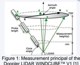
Figure 1: Measurement principle of the Doppler LIDAR WINDCUBE™ V1 [1]
