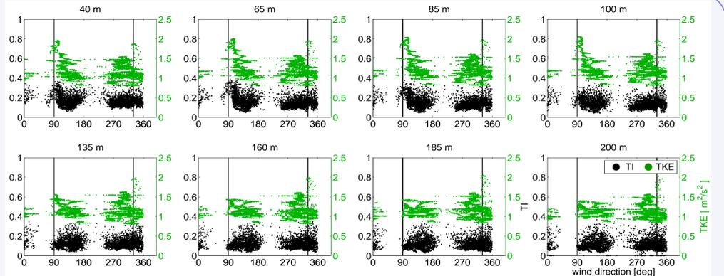
Figure 4: TI and TKE plotted in black and green as a function of wind direction, using the turbulence processed data set for wind speeds  $> 3$  m/s. The vertical black lines at  $90^\circ$  and  $330^\circ$  indicate disturbed winds due to the wakes of WEA4 and WEA5.
