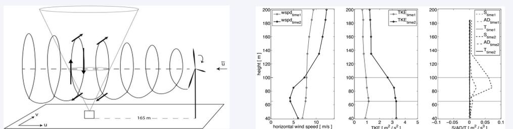
Figure 6: a) Sketch of the wake structure and derived wind pattern captured by the device. b) Vertical profiles of wind speed, TKE and TKE budget terms for time1 = 00 CET and time2 = 09 CET on September 25th 2010. Horizontal heights indicate the blade tip and hub height.
