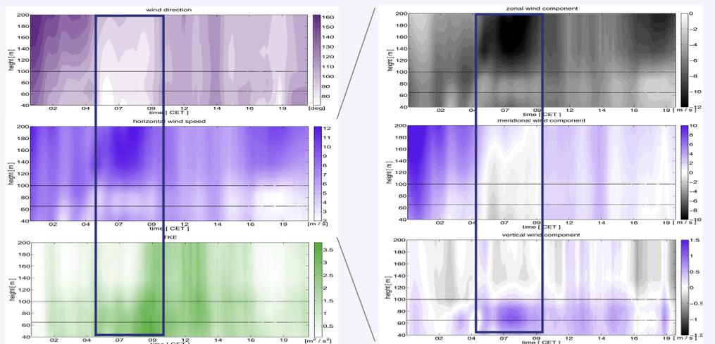
Figure 5: Contour plots of wind direction, horizontal wind speed, TKE (left) and wind components  $u$ ,  $v$  and  $w$  (right) profiles during the wake case of September 25th 2010. The purple boxes and black horizontal lines indicate the period during which the device was inside the wake region and hub and blade tip height respectively.
