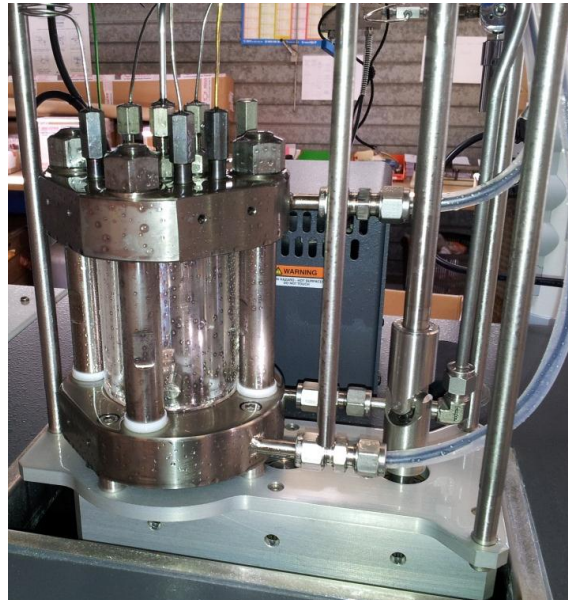
Phase equilibrium cell under pre-acceptance test (Source: SINTEF)
