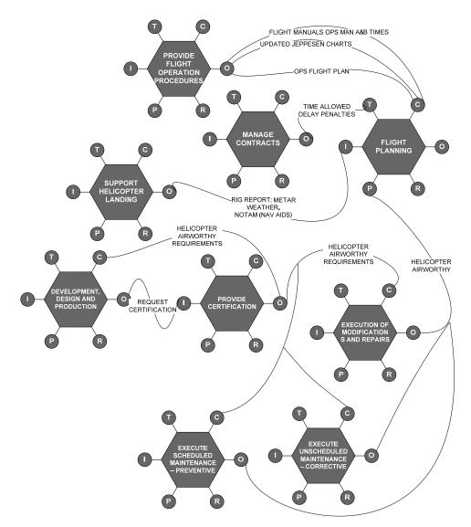
Figure 9.2. Selected elements of FRAM for scenario landing on helideck.
