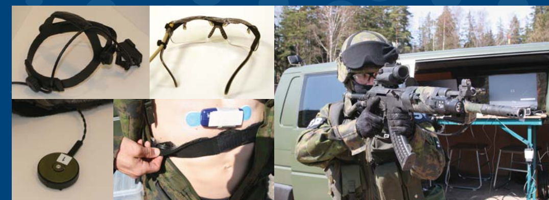
Fig.2. The wearable UI: a head-mounted display, LED glasses, tactors, and the ECG device
