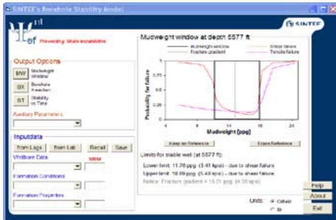
PSI estimates the probability for mechanical failure inside the borehole wall; since the model is largely analytical, solutions are obtained very quickly. The software allows for analysis of stresses and pore pressure around the considered well and analysis of stability versus time since drilling.
