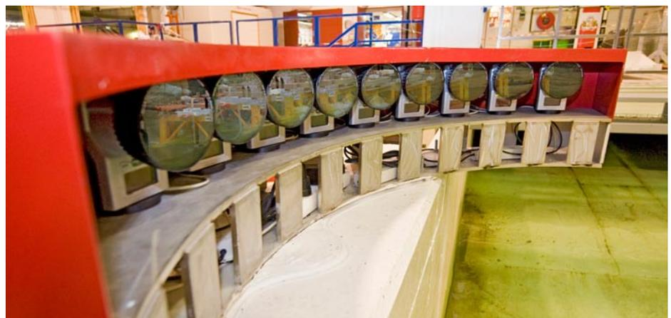
Figure 1. New Oqus position measurement cameras in the Ocean Laboratory.
