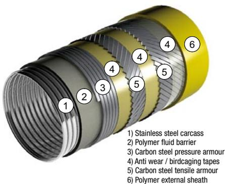
*Cross-section of a flexible riser, showing the most important layers of the wall structure.*
