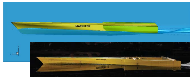
Figure 2: Trimaran, 35 knots. Wave pattern. Comparison with model tests.
