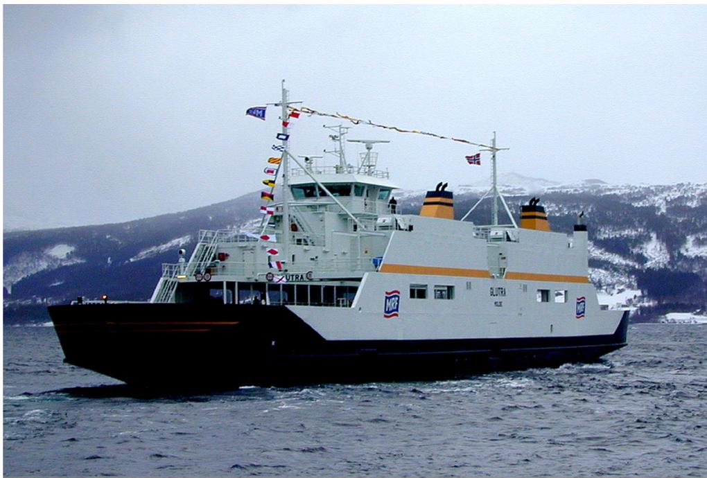
**Figure 1** “Glutra” – The first natural gas engine powered ferry in the world with “gas-electric” propulsion system.
